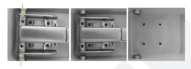
7 – Once you have removed the closing handle, replace it with a new handle and secure it in the reverse order to what is described above: place the closure in the specific seat and slide the upper and lower slots inserting them in the closure seat.
