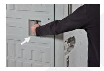
2. With the right hand, grasp the handle in a position corresponding to the black lever, pushing it slightly forward.
