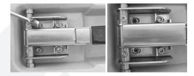
4 - Remove the two stainless self-locking hex nuts M6 on the rod and pull out the two stainless steel countersunk hex head screws M6x25
