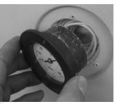
2 - Enter a new thermometer, taking care to place the bulb of the probe in a position corresponding to the holes on the probe cover plate and tighten the three stainless steel self-tapping screws 3.9 X 16mm with cylindrical head and cross cut.
