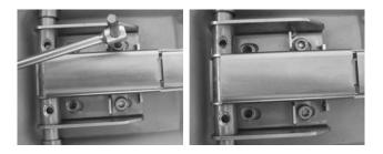
9 - Insert on the rod the two stainless steel countersunk hex head screws M6x25 and tighten the two stainless steel self-locking hex nuts M6.
