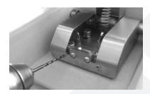
2 – Remove the metal cover using a flat tool (e.g.: slotted screwdriver)
