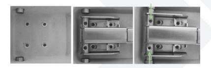
8 - Screw the 2 stainless steel socked head cap screws M8x16 with stainless steel groover washers (screws located externally, on the right).
