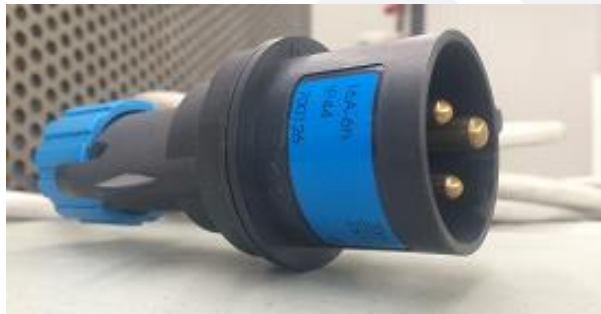
Picture 3 - blue IEC309 plug (2 poles + 230V 16A earth) for connection to the 230Vac 50-Hz power supply
